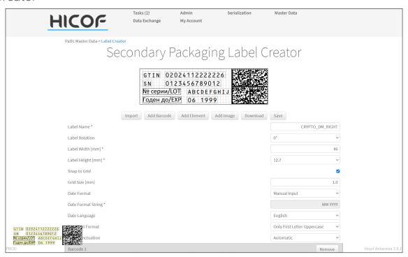
Hicof AMACENA features a build-in web based label creator to create and adjust all print layouts for AMACODERS, and all connected tertiary label printers. The label creator allows GMP compliant change control of all label parameters across the enterprise.
